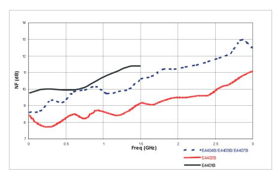
Nominal Instrument Noise Figure 3 to 26.5 GHz No Preamplifier; two example units
